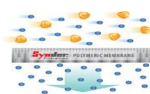
Cross Flow Filtration
