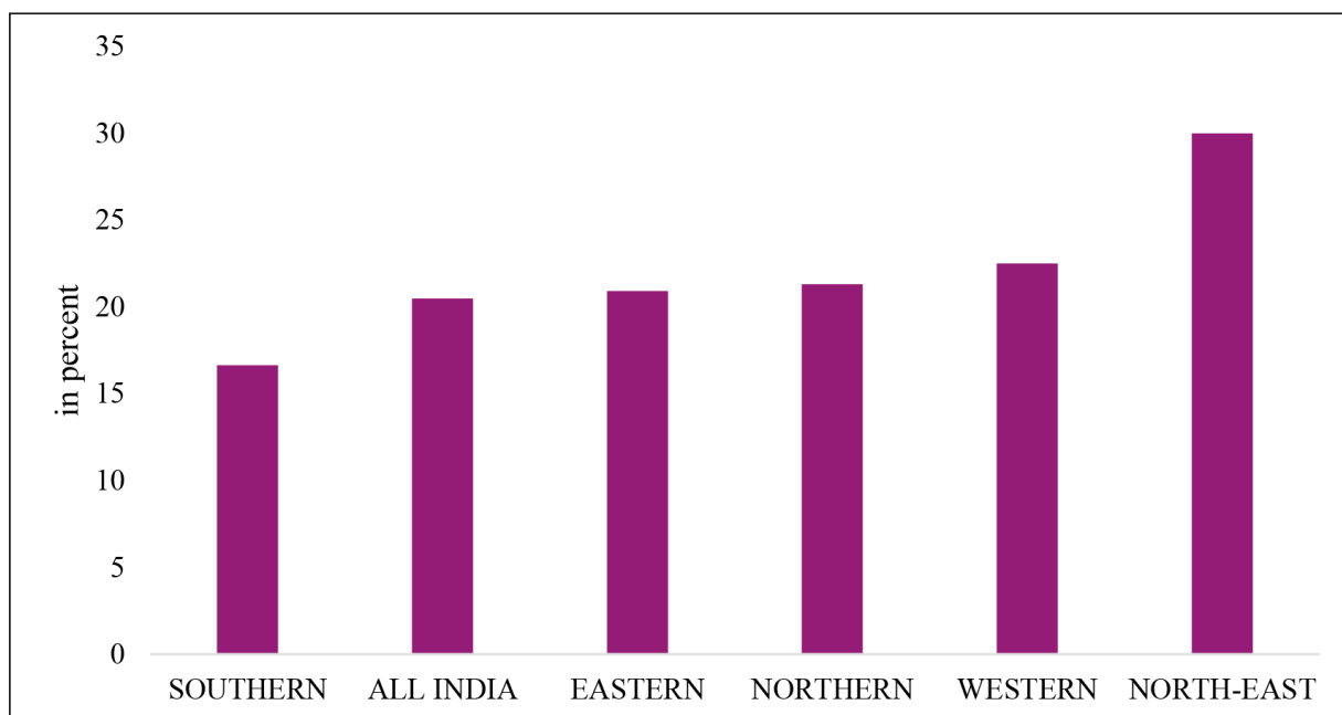
Figure 45: Energy loss in transformation, transmission and distribution and unaccounted for as a percentage of Net energy available for supply
